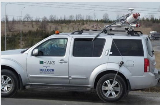
Figure 41 – LiDAR high speed street lighting luminaire and pole survey vehicle (Haks Inc)
